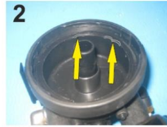
2 LOCATE ON THE MOUNTING BASE THE CUTS FOR THE SINGLE AND THE DOUBLE NOTCHES
